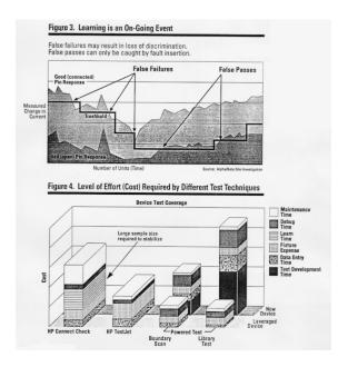
Using a learned threshold to distinguish defects results in a significant amount of maintenance and adjustment time after the technique is in production, with a widely variable false pass rate. The tradeoff is in the ability to
